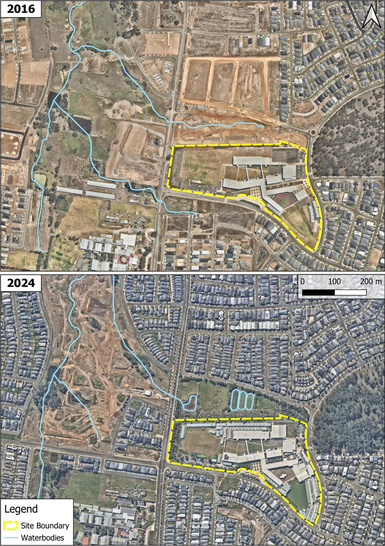
Figure 4: Development and watercourse reconfiguration surrounding the site between 2016 and 2024 (Source: Nearmap)
