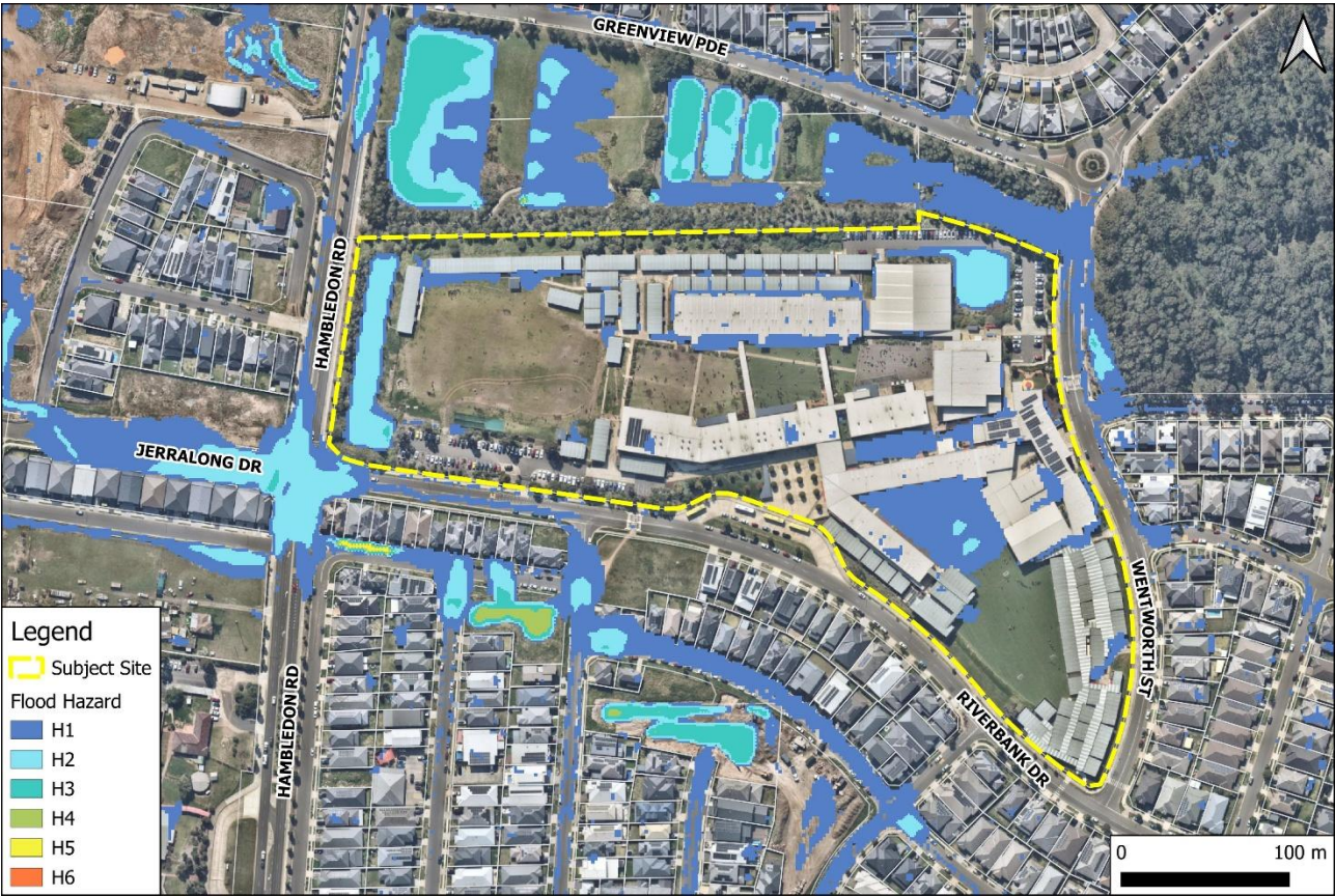
50% AEP event – flood hazard classification surrounding the site – Pre-Development Scenario
