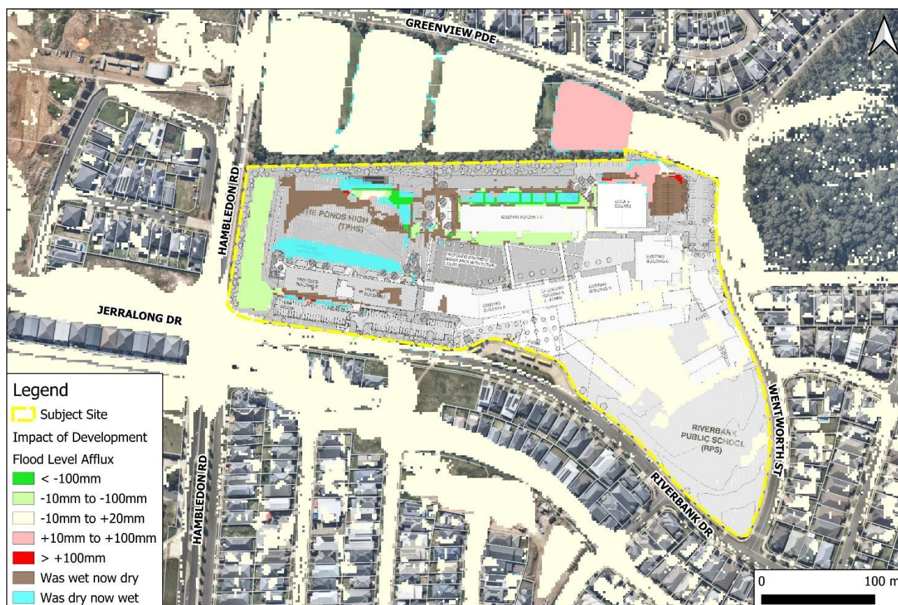
Figure 35: 0.2% AEP Flood Level Impact (Post-Development Scenario – Pre-Development Scenario)
