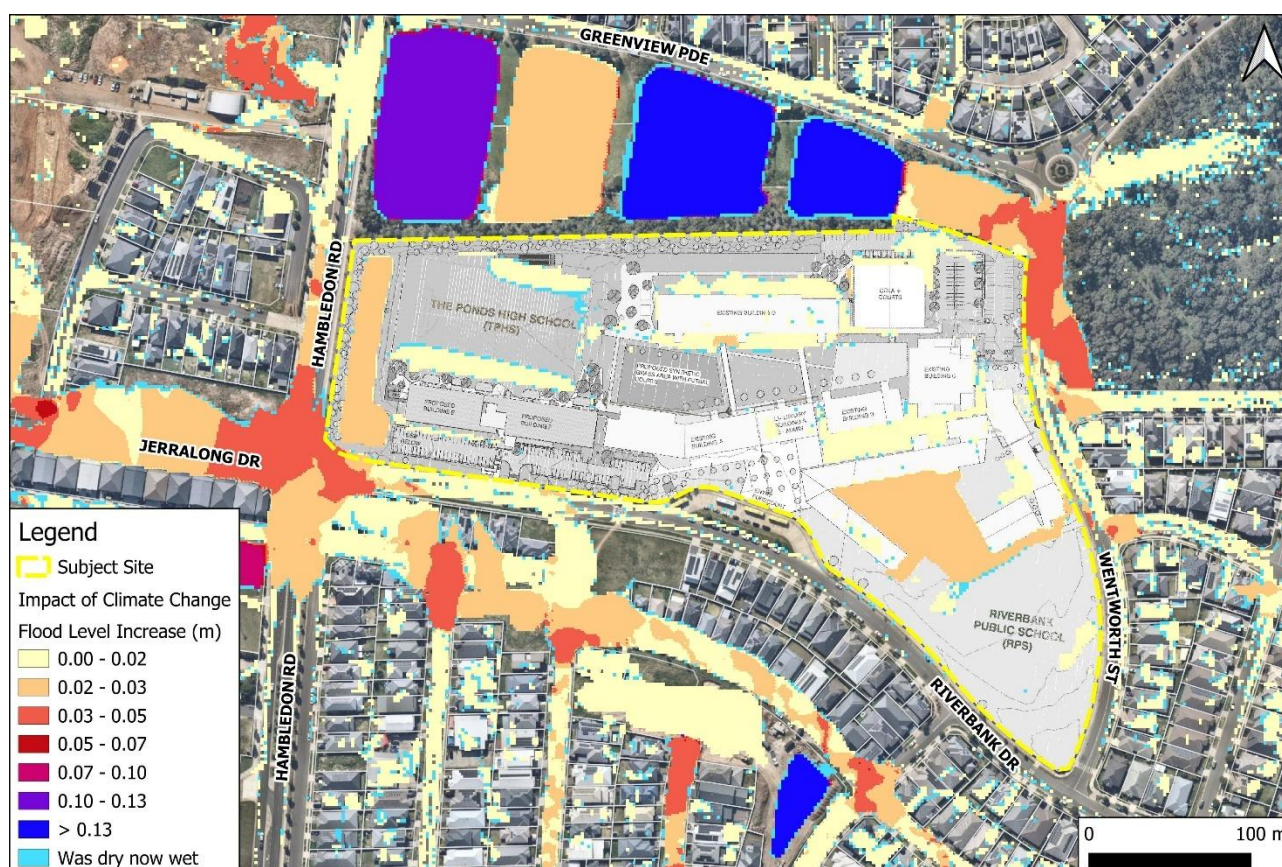
Figure 36: 1% AEP flood level afflux (m) under the adopted 2090 climate change scenario (Post-Development Scenario)
