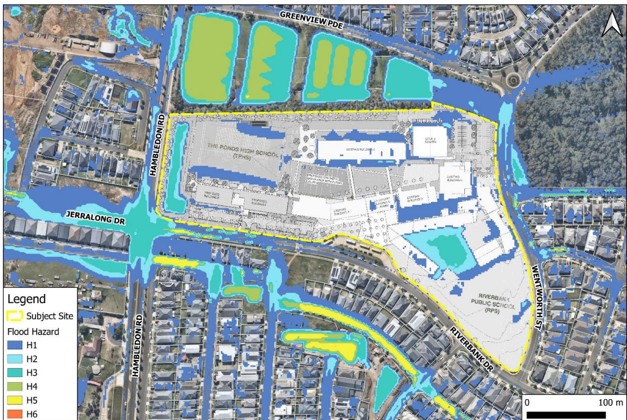
Figure 30: 1% AEP event – flood hazard classification surrounding the site – Post-Development Scenario
