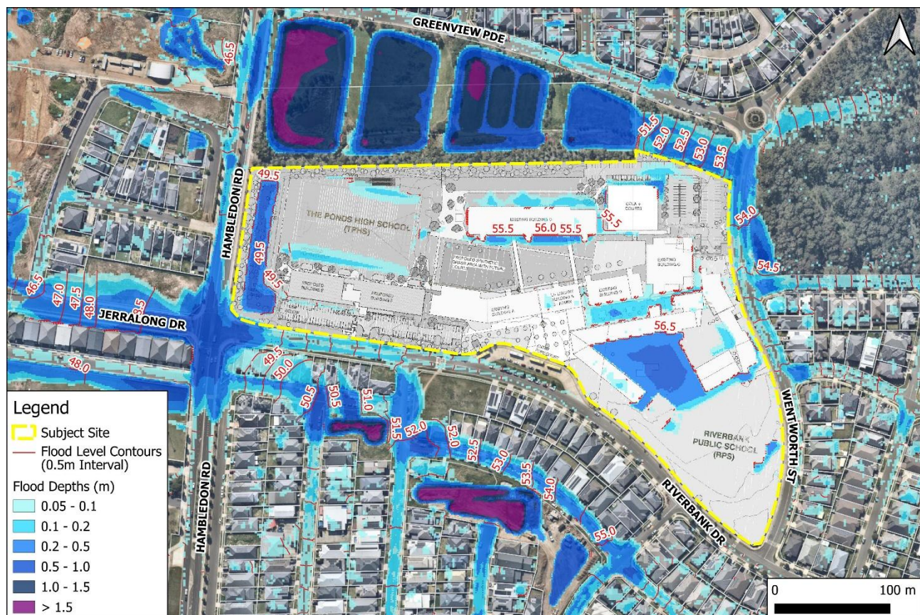
Figure 28: 1% AEP event – flood depths and levels surrounding the site – Post-Development Scenario
