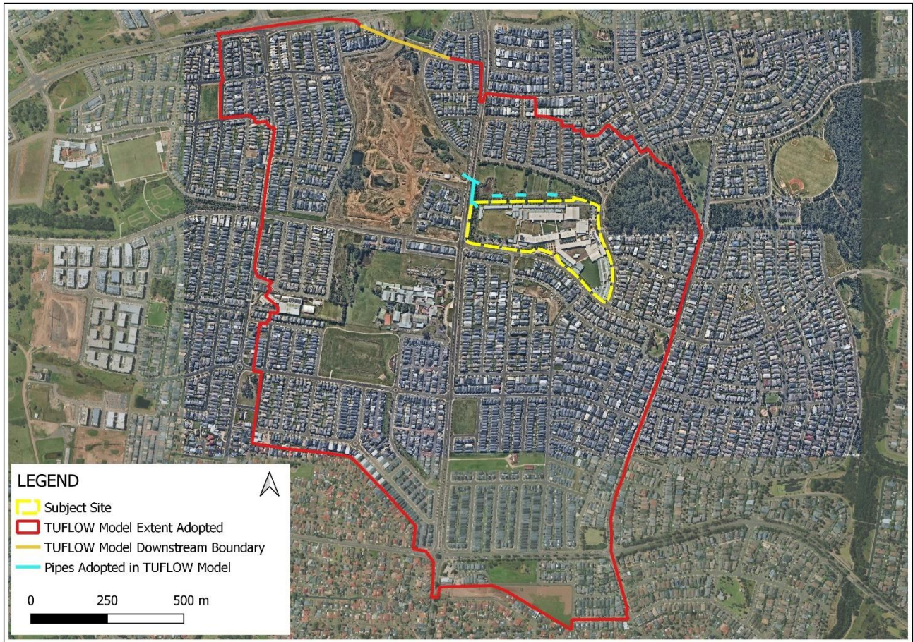
Figure 12: TUFLOW model extent and downstream boundary adopted
