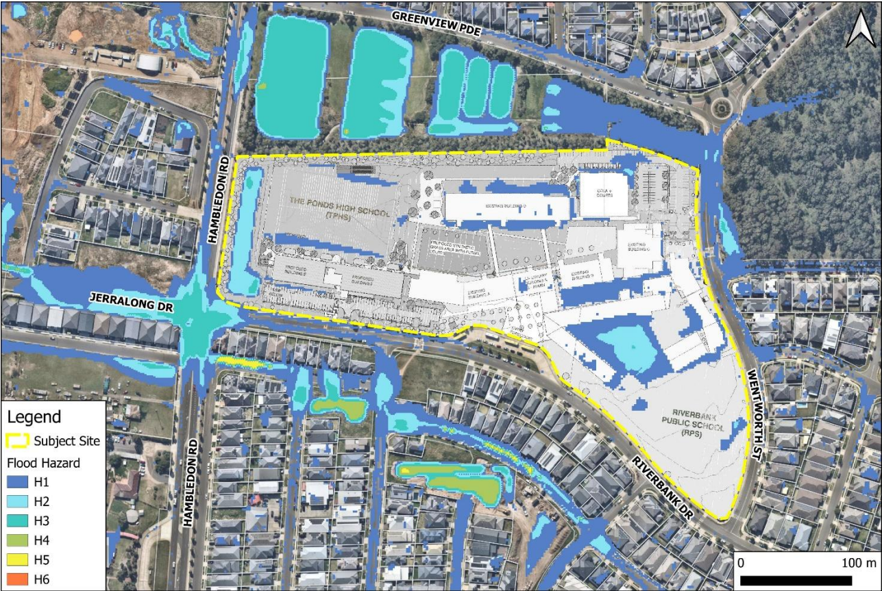
Figure 27: 10% AEP event – flood hazard classification surrounding the site – Post-Development Scenario
